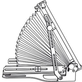
⑤ Screw front standard into desired base mount (see page 9 for guidance).
