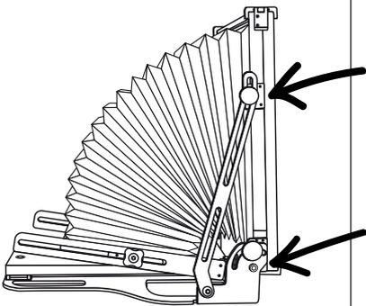
④ Raise front standard and tighten rise / fall controls.
