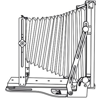
③ Lock rear standard at 90° to zero and tighten both sets of screws.
