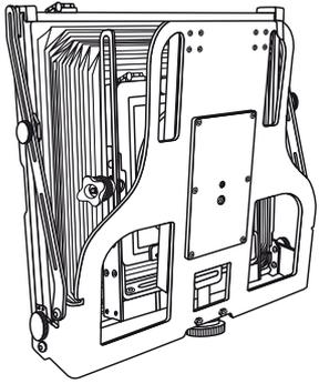
② Loosen rear standard screws and raise the rear while pulling front forwards.
